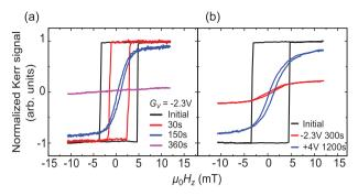
**Figure 4.** pMOKE hysteresis loops measured in sample S3 (350  $^{\circ}$ C, zero dwell time) showing an SRT induced by the exposure to a gate voltage of -2.3 V for a) 360 s, and b) partial reversibility of the IP magnetized state after exposure to +4 V for 1200 s.
