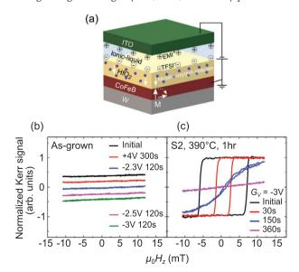
**Figure 1.** a) Schematic of the structure of the ionic-liquid gate device and pMOKE signal under an out-of-plane magnetic field ( $\mu_0H_z$ ) of the b) as-grown, and c) annealed S2 sample under different gate voltages and gating times.
