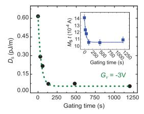
**Figure 2.** Surface DMI constant  $(D_s)$  as a function of the gating time under a gate voltage  $G_V = -3$  V in sample S2. The inset shows the corresponding changes in  $M_s \cdot t$ , where  $M_s$  is the saturation magnetization and t the thickness of the film, respectively. The error bars represent the noise amplitude of the measurement. The dotted lines are a guide to the eye.
