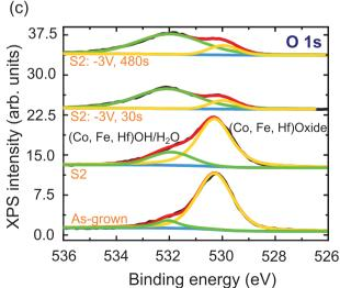
**Figure 3.** XPS spectra of a) Fe  $2p_{3/2}$  and  $2p_{1/2}$ , b) Co  $2p_{3/2}$  and  $2p_{1/2}$ , and c) O 1s for as-grown samples, S2, and S2 exposed to -3V for 30 and 480 s. Raw data (black), total fitting (red), background (blue), and fitting of each peak: light green and yellow for O 1s peaks; dark green for Co and Fe 2p, and purple (dashed and solid) for oxides of Fe and Co 2p.
