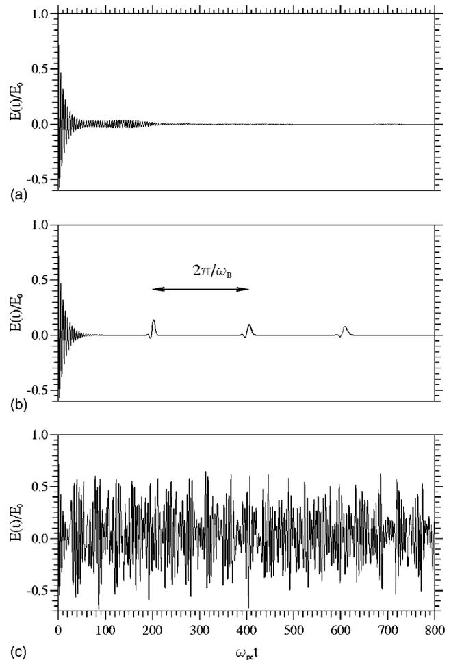
FIG. 6. Time evolution of the electric field  $E(t)/E_0$  as a function of normalized time for  $A=0.03$ ,  $k=0.405$ , and, respectively,  $\gamma=5.77 \times 10^{-3}$  (a),  $\gamma=0.173$  (b), and  $\gamma=1.155$  (c).
