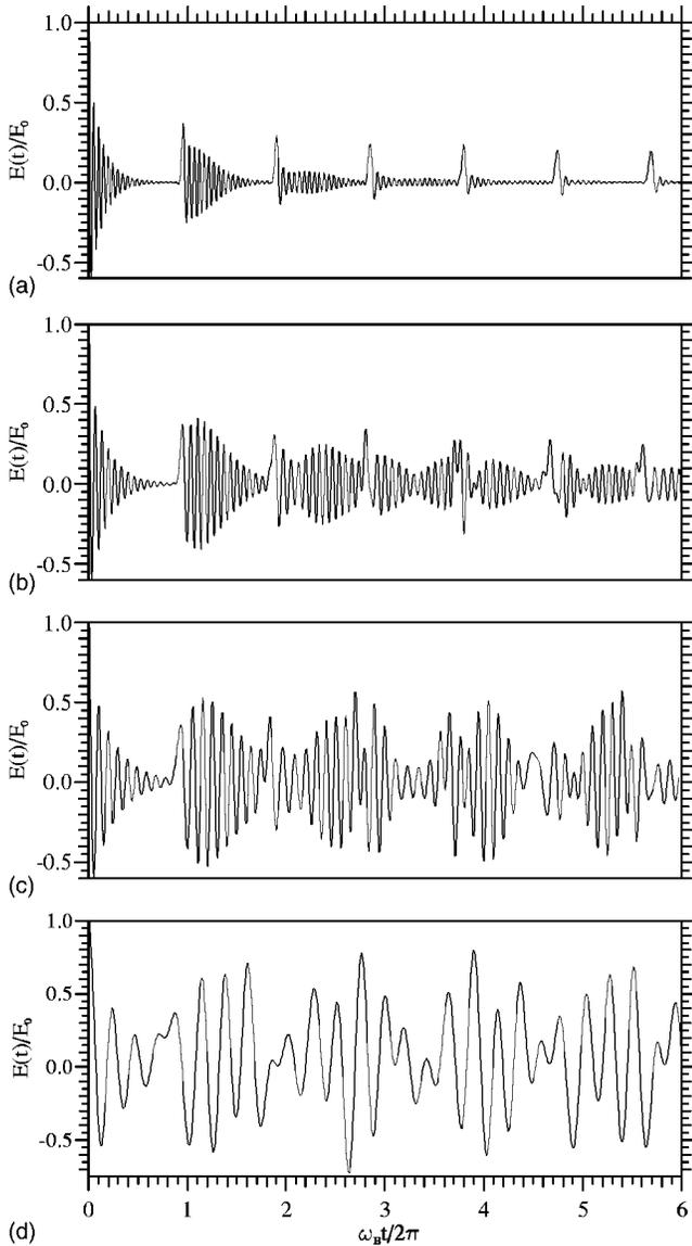
FIG. 3. Time evolution of the electric field  $E(t)/E_0$  as a function of time normalized to the electron cyclotron period for  $\gamma=0.629$  (a),  $\gamma=0.85$  (b),  $\gamma=1.25$  (c), and  $\gamma=3$  (d).  $A=0.01$  and  $k=0.405$ .
