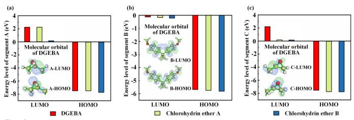
Figure 5. The changes in LUMO and HOMO energy levels of different segments of DGEBA, chlorohydrin ether A, and chlorohydrin ether B molecules. (a): Segment A; (b): Segment B; (c): Segment C
