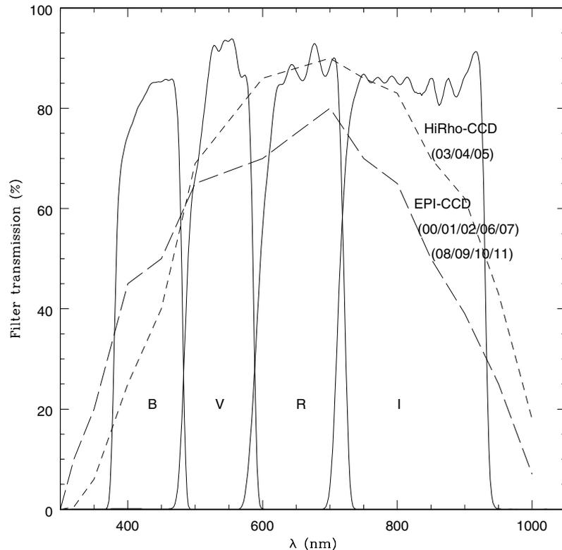
**Fig. 2.** Filter transmission and CCD quantum efficiency of the CFH12K camera used for the VIRMOS optical survey. The camera is composed of 9 epitaxial silicon (EPI) and three high resistivity (HiRho) devices. Both devices have different quantum efficiency, as show by the long-dashed and short-dashed curves. The numbers indicate the CFHT reference number of the CFH12K CCDs.
