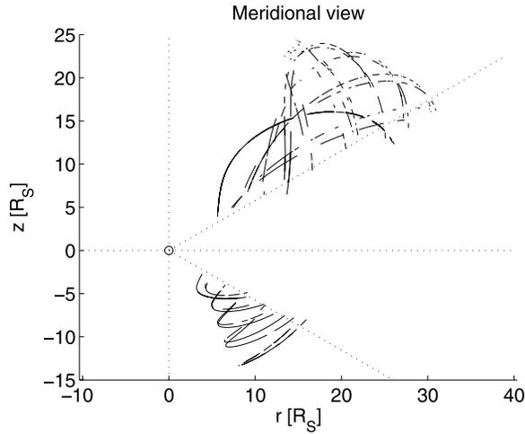
**Figure 9.** Position of Cassini during occurrence of elliptically polarized SKR from September 2006 until May 2007 in meridional view. Saturn's rotation axis ( $z$  axis), its equatorial plane ( $z = 0$ ), and the latitudes of  $\pm 30^\circ$  are indicated by dotted lines.
