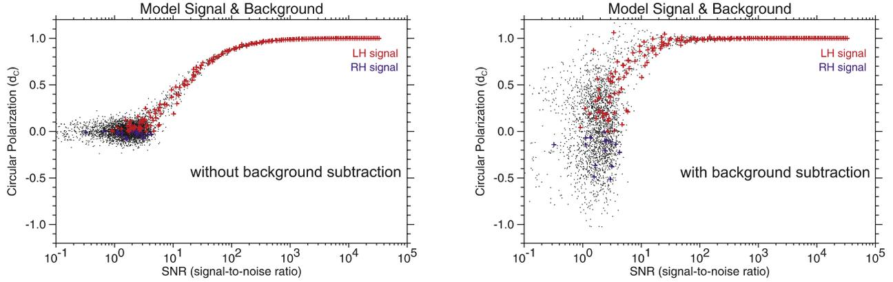
**Figure B1.** Model calculation of the degree of circular polarization  $d_c$  for all spectral points (black dots) and signal points (red or blue plus signs) as a function of signal-to-noise ratio (SNR). The incoming wave direction is the  $-y$  direction in the Cassini s/c-frame. For the modeled autocorrelations we plot the case of (left) no background subtraction and (right) with the subtraction of the 5% occurrence level background.
