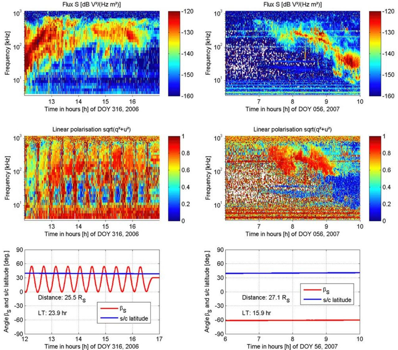
**Figure 6.** Two examples of flux and linear polarization spectra retrieved from RPWS three-antenna direction finding showing elliptically polarized SKR. At the bottom the spacecraft latitude as well as the angle  $\beta_S$  between the center of Saturn and in this case the  $E_u$ – $E_w$  antenna plane are given. Additionally the mean spacecraft distance and local time are noted, which both do not change significantly within the respective time interval.
