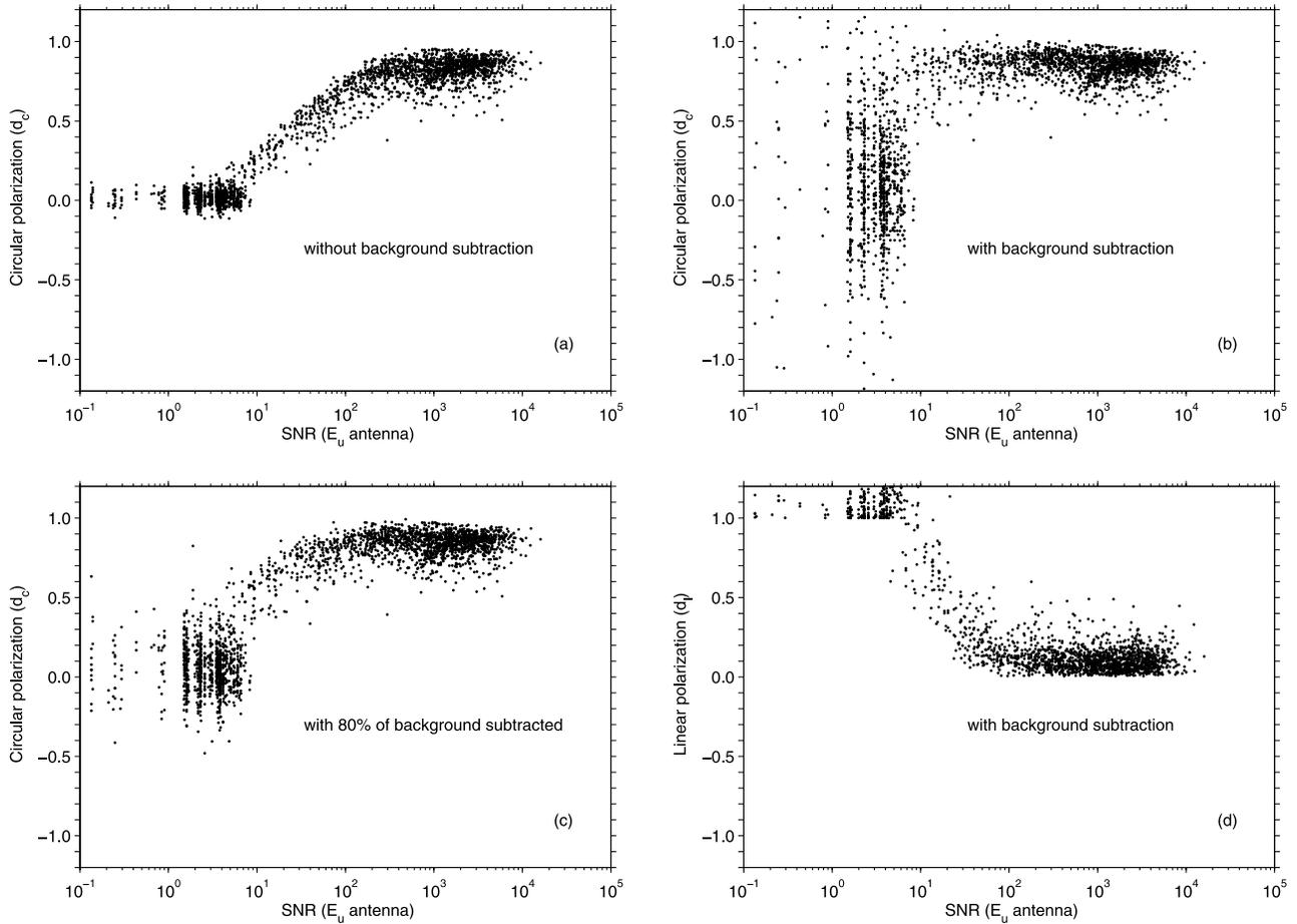
**Figure B2.** Circular polarization  $d_c$  and linear polarization  $d_l$  as a function of signal-to-noise ratio (SNR) of RPWS data from DOY 197, 2004, 10–11 SCET in the frequency interval from 45 to 975 kHz. The four panels show (a)  $d_c$  in case without a background subtraction, (b)  $d_c$  in case with background subtraction, (c)  $d_c$  for subtracting only 80% of the background (from the autocorrelations before the DF inversion), and (d)  $d_l$  in case with background subtraction.
