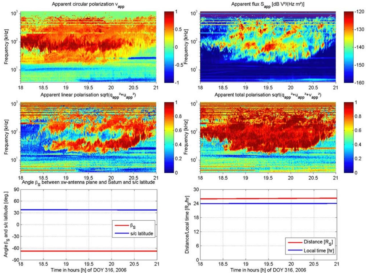
**Figure 4.** Apparent polarization spectra and orbital parameters of Cassini similar to Figure 3. The time goes from 18 to 21 SCET on DOY 316, 2006 and from the high apparent linear polarization at the constant angle of  $\beta_S = -66^\circ$  the real elliptical polarization of SKR is evident.
