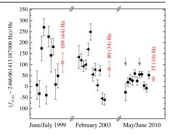
FIG. 5 (color online). The 1S–2S centroid frequency of the current measurement is compared with the previous two measurements [3,7]. The filled points represent an average per day, the open points (with label) are the final values. Their error bars represent the total  $1\sigma$  uncertainty. The arrows indicate the measurements directly after refreshing the graphite coating of the excitation region and of the Faraday cage.
