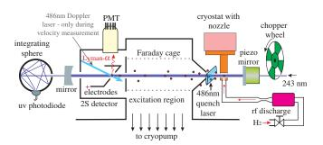
FIG. 1 (color online). Schematic of the beam apparatus. A standing laser wave at 243 nm (between gray mirrors) with a  $1/e^2$  waist radius of  $w_0 = 292 \ \mu m$  at the flat cavity front mirror excites the sharp 1S-2S transition in a collinearly propagating cold thermal beam of atomic hydrogen emerging from a cooled copper nozzle. The 2S state is detected after quenching with a localized electric field which releases a Lyman- $\alpha$  photon. See text for further details.
