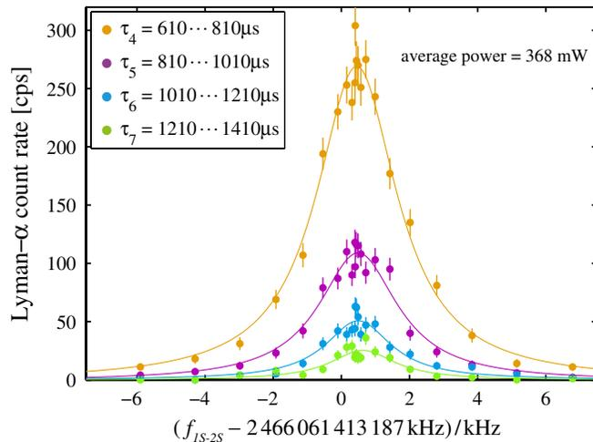
FIG. 2 (color online). Single scan line profile for different delays along with Lorentzian fits. With the detection delay  $\tau$ , we set an upper limit on the atoms velocity but reduce the signal accordingly. The full width at half maximum (FWHM) is about 2 kHz.
