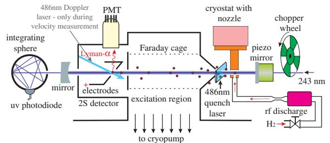
FIG. 1 (color online). Schematic of the beam apparatus. A standing laser wave at 243 nm (between gray mirrors) with a  $1/e^2$  waist radius of  $w_0 = 292 \mu\text{m}$  at the flat cavity front mirror excites the sharp 1S–2S transition in a collinearly propagating cold thermal beam of atomic hydrogen emerging from a cooled copper nozzle. The 2S state is detected after quenching with a localized electric field which releases a Lyman- $\alpha$  photon. See text for further details.
