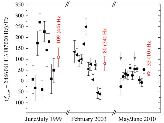
FIG. 5 (color online). The  $1S-2S$  centroid frequency of the current measurement is compared with the previous two measurements [3,7]. The filled points represent an average per day, the open points (with label) are the final values. Their error bars represent the total  $1\sigma$  uncertainty. The arrows indicate the measurements directly after refreshing the graphite coating of the excitation region and of the Faraday cage.
