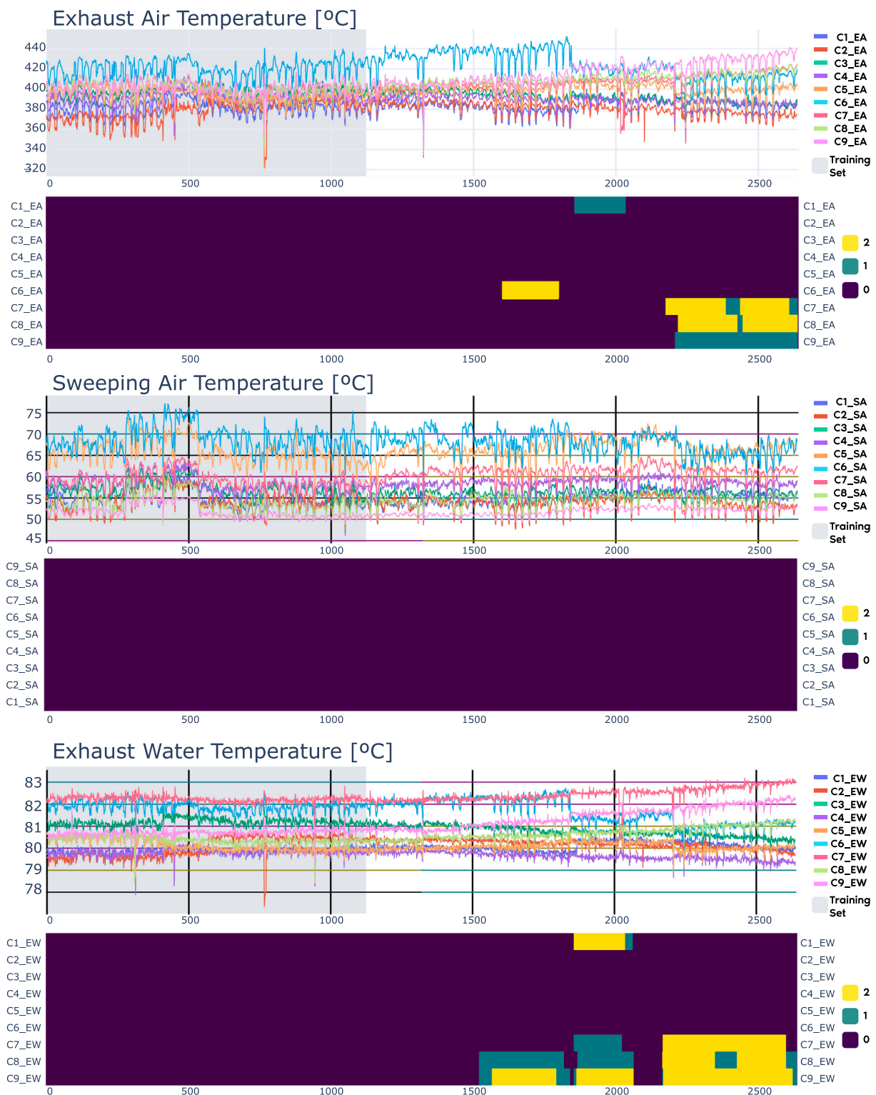
Fig. 16. Results obtained through SDTs. The anomaly score (0,1,2) corresponds to the variation registered in the feature-slope within anomalous behavior conditions.
