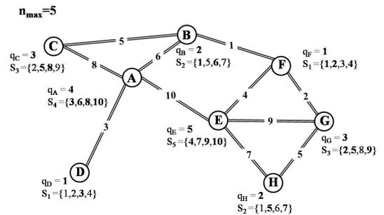
Fig. 3. Example of channel assignment ( $n_{max} = 5$ ). The precised number on every link denotes the common dedicated data channel.
