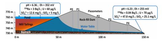
Fig. 1. Cross section through the dam and water chemistry along the flow path (measurements of October 2006) according to Combes and Schmitt [3].
