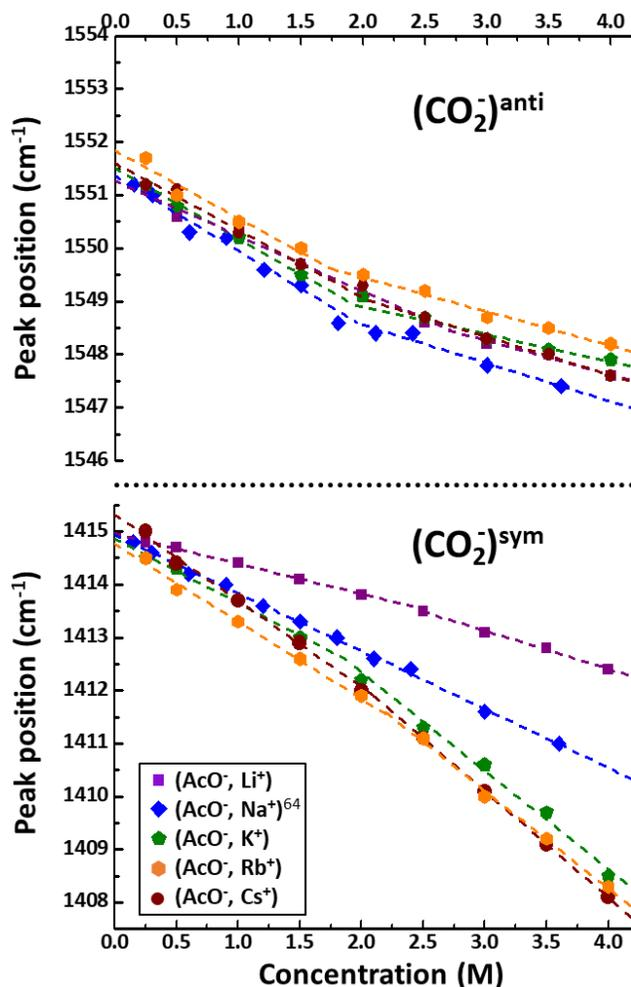
**Fig. 1** Peak position of the  $(\text{CO}_2^-)^{\text{sym}}$  (down) and  $(\text{CO}_2^-)^{\text{anti}}$  (top) transitions of ATR-FTIR spectra presented in Fig. S4, as a function of concentration. Dotted lines are the best linear fit passing through low and high concentration subsets.
