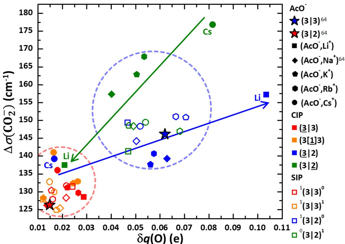
**Fig. 7** Frequency splitting of the carboxylate stretching modes  $\Delta\sigma(\text{CO}_2^-)$  as a function of the unsigned charge difference between both oxygen atoms of carboxylate  $\delta q(\text{O})$ , determined by NBO analysis at the RI-B97-D3/dhf-TZVPP level, for all coordination types of each cluster. Dashed circles represent two sets with different coordination types: the symmetric coordination types  $3|3$  in orange and the asymmetric coordination types  $3|2$  in blue. The blue
