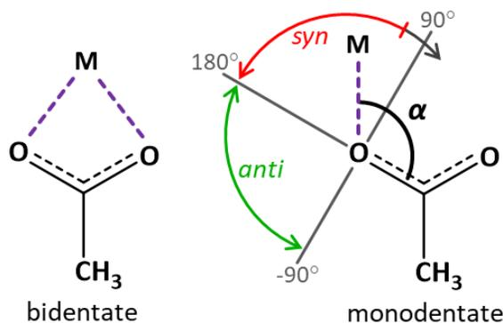
**Fig. 4** Binding geometries and naming conventions for metal ion carboxylate adapted from Carrell *et al.*,<sup>[68]</sup> where  $\alpha$  is the  $C_{\text{carboxylate}}\text{-O}\cdots\text{M}^+$  bond angle projected onto the carboxylate plane. Note that *syn*-monodentate type of binding lies in the  $\alpha=[100^\circ, 180^\circ]$  range, *anti*-monodentate lies in the  $[-180^\circ, -90^\circ]$  range, and bidentate binding lies in the  $[80^\circ, 100^\circ]$  range.
