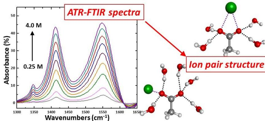
ATR-FTIR spectra of acetate alkali-metal solutions display a cation-dependent behavior which can be correlated to ion pair formation. Simulations in explicit solvent and frequency calculations are used to identify the main supramolecular structures present in solution.
