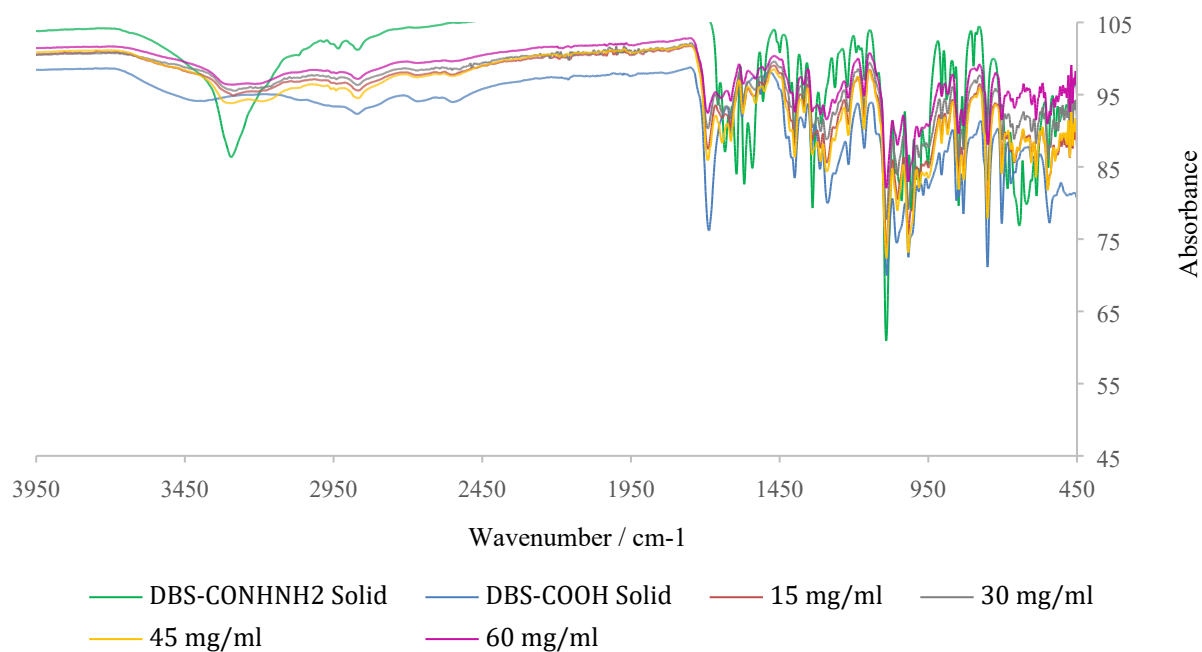
Figure S18. IR Spectra of DBS-COOH solid (blue), DBS-CONHNH 2 solid (green) and DBS-COOH/DBS-CONHNH 2 multicomponent gel filaments: 1.5% wt/vol (red), 3.0% wt/vol (grey), 4.5% wt/vol (yellow) and 6.0% wt/vol (purple).
