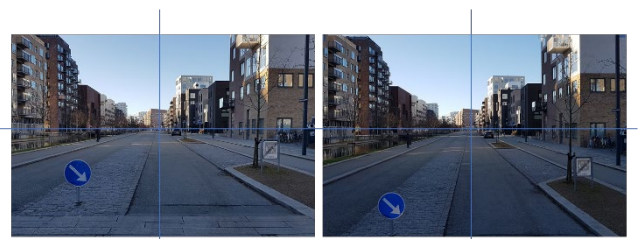
Figure 3: Car and truck driver perspectives at same location. Note the different convergence of curb lines, and how the horizon line intersects windows and vertical posts at different heights.
