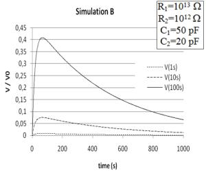
Fig. 6. Simulated return voltage using the two-cell RC model.
