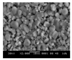
Fig. 4. SEM photograph of the alumina plates surface [14]
