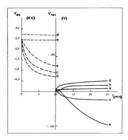
Fig. 9. Anomalous return voltage on polyethylene [7].
