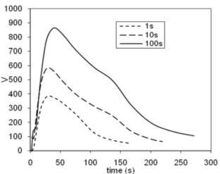
Fig. 5. Return voltage measurements on 1mm-thick polycrystalline Al2O3 slabs previously polarized at 2500V (during 1s, 10s, 100s). [14].
