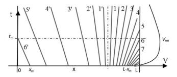
Fig. 8. Charge sheets motion on both sides of the zero-field plane (left and center of the figure) during the voltage return experiment (voltage shown on the right). Charge sheets are numbered according to the distance to the zero field plane (dotted line), N and N' referring to charges subjected to the same absolute value of the field.
