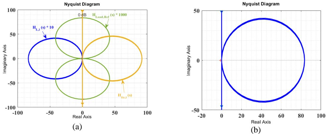
Fig. 4: The step response-based Nyquist diagrams of (a) each transfer function in (21), and (b) transfer function (20).
