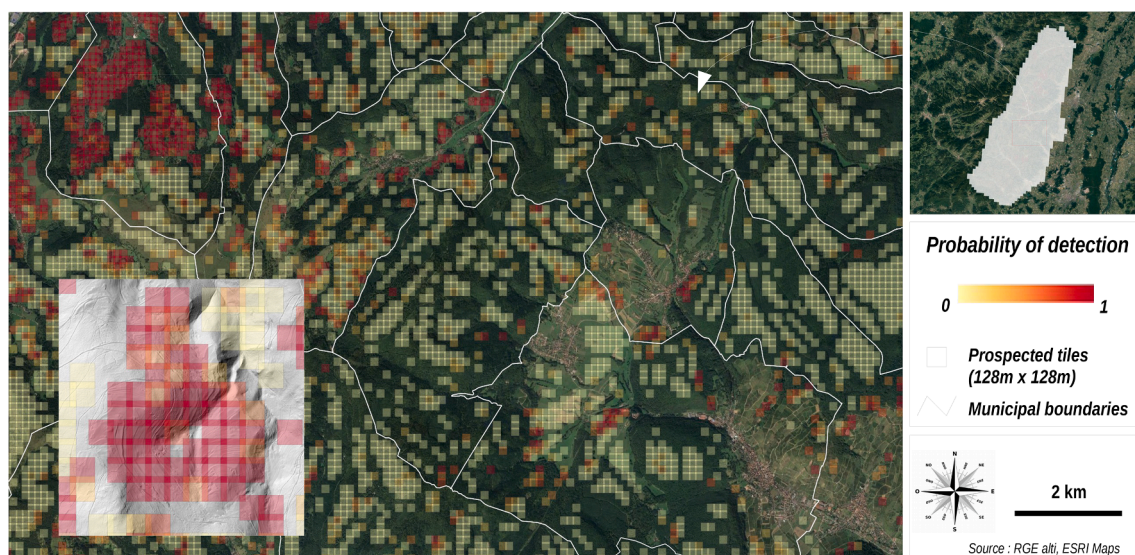
Fig. 9. Example of TS probability map generated through the properties of the FCN model decision process.
