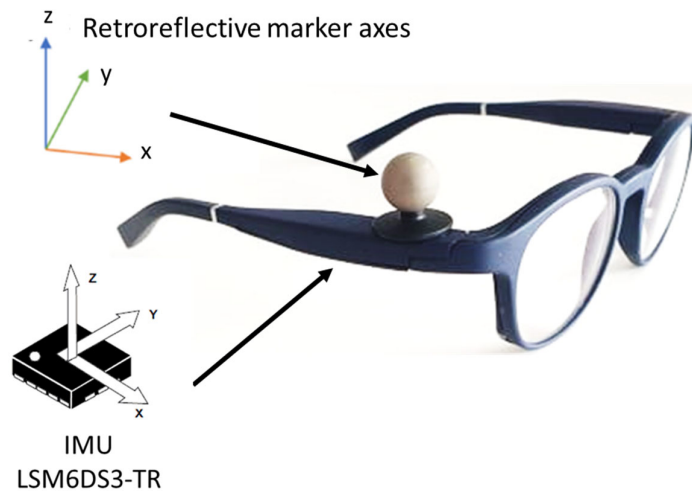
Figure 2. Position of the retroreflective marker on the right arm of the glasses and axes of the IMU and retroreflective marker.
