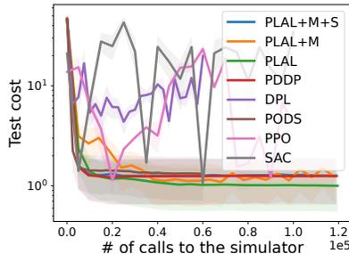
Fig. 3. **Sample efficiency: constrained LQR.** Model-based methods outperform model-free RL on tasks with linear dynamics and a stable target. We also evaluate the impact Sobolev training (+S) and multiple shooting (+M) or removing the constraint handling (-C).
