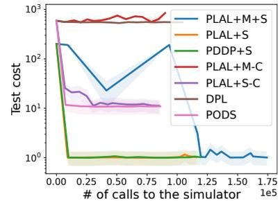
Fig. 4. **Sample efficiency: inverted pendulum.** Using a constrained formulation (5) along with supervision of the derivatives appears essential to reach a precise solution on a non-linear dynamics with unstable target.
