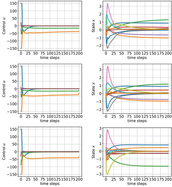
Fig. 6. **Comparisons of controllers from TO and policy learning.** We represent the trajectories (**right**) and the corresponding control (**left**) on a testing sample of UR5. The 1<sup>st</sup> row corresponds to the learned policy while the 2<sup>nd</sup> and 3<sup>rd</sup> represent the trajectories obtained via TO when the solver is initialized respectively with and without the learned controller.
