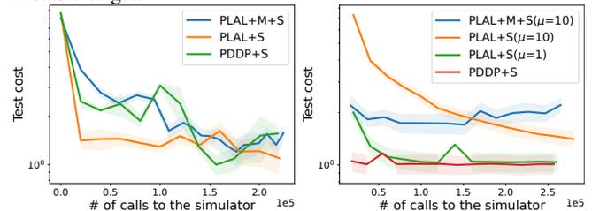
Fig. 5. **Samples efficiency: robotics tasks.** Due to chaotic dynamics, the double pendulum (left) and UR5 (right) require both handling constraints and the Sobolev training to converge. When it is so, it converges quickly towards a precise solution. Even though policy parameters are identically initialized across the different algorithms, on UR5 the first test evaluations are only performed after a few training steps to avoid numerical divergence during rollouts.
