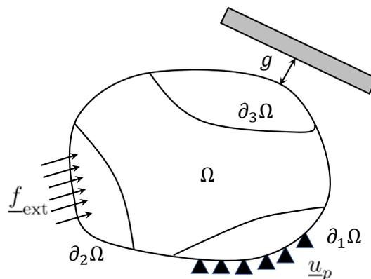
Figure 1: Frictional contact problem setting.
