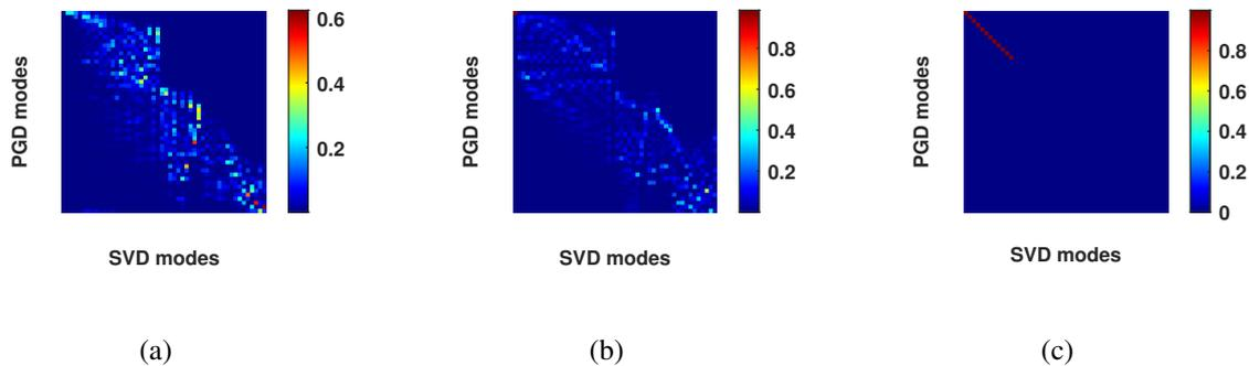
Figure 11: MAC diagrams for space modes  $\mathbf{W}$ : (a) with orthonormalization, (b) with orthonormalization and time function update, (c) with downsizing.
