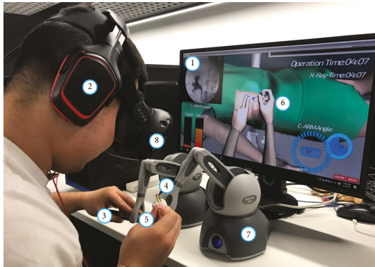
Fig. 3: Simulator for renal biopsy based on Touch interfaces [14]
