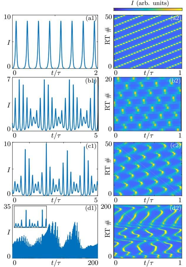
Figure 2: Time-domain simulations of (1) for  $A = 2.7$  and  $\tau = 335$ , showing intensity time series (left, a1-d1) and their pseudo-space representation (right, a2-d2); here  $\kappa = 0.007$  in (a),  $\kappa = 0.0159$  in (b),  $\kappa = 0.04$  in (c), and  $\kappa = 0.1$  in (d). The inset in panel (d1) shows an enlargement of the intensity time series over two roundtrips in the external feedback cavity.
