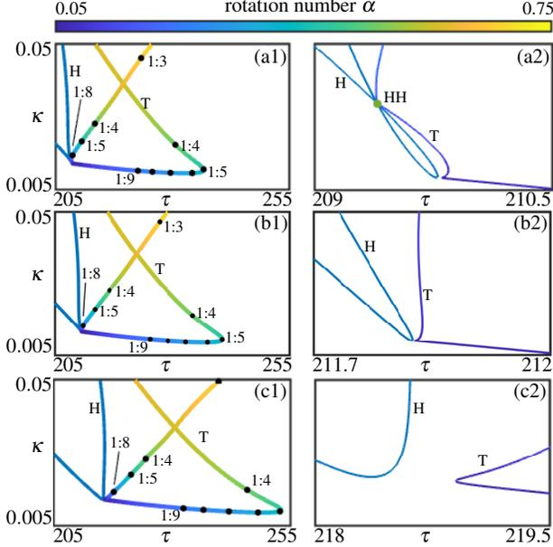
Figure 6: Bifurcation diagram in the  $(\tau, \kappa)$ -plane illustrating the disappearance of the Hopf-Hopf bifurcation point HH from Figure 5 for  $A = 2.39$  (a),  $A = 2.38$  (b) and  $A = 2.35$  (c). Panels (a1)–(c1) show a larger view of the Hopf bifurcation curve H and the torus bifurcation curves T, where the rotation number  $\alpha$  along T is indicated according to the color bar and low-order resonance points are marked. Panels (a2)–(c2) are further enlargements.
