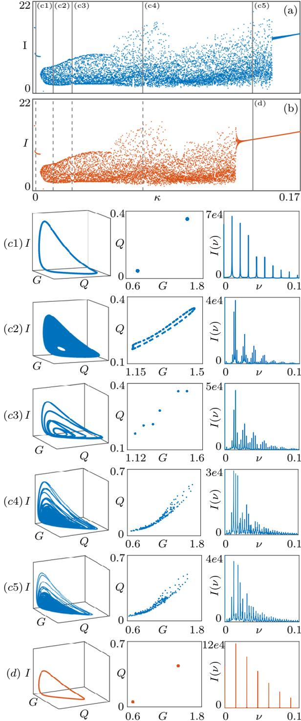
Figure 3: One-parameter bifurcation diagrams of (1) for  $A = 2.7$  and  $\tau = 335$  where  $\kappa$  is increased (a) and decreased (b). Also shown are representative trajectories in  $(G, Q, I)$  space (left), their intersection with a Poincaré section represented by the  $(G, Q)$ -plane (middle), and corresponding RF spectra (right), for  $\kappa = 0.002$  (c1),  $\kappa = 0.013$  (c2),  $\kappa = 0.025$  (c3),  $\kappa = 0.07$  (c4) and  $\kappa = 0.14$  (c5,d).
