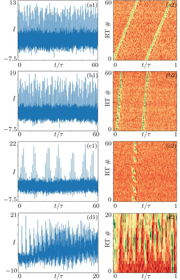
Figure 1: Experimental intensity time series (left, a1-d1) and their pseudo-space representation (right, a2-d2) for: (a) equally spaced two pulses per feedback roundtrip ( $\tau = 5.47$  ns), (b) symmetry-broken two pulses per roundtrip ( $\tau = 8.22$  ns), (c) modulated quasiperiodic regime ( $\tau = 4.78$  ns), and (d) complex dynamics above the lasing threshold ( $\tau = 4.77$  ns).
