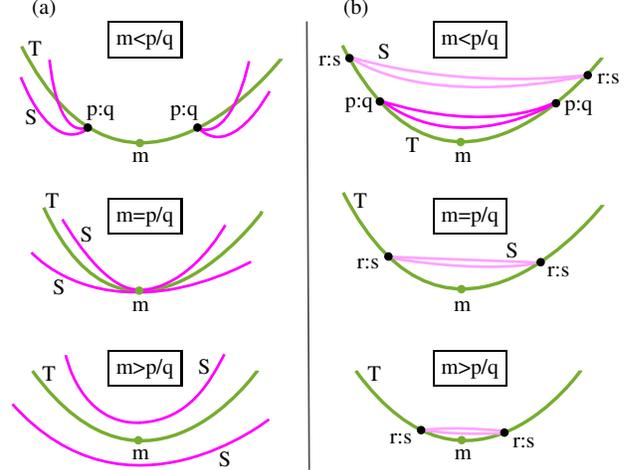
Figure 9: Sketches of the two scenarios for disconnecting (a) and disappearing (b)  $p:q$  resonance tongues near an extremum of the rotation number on a curve T of torus bifurcation. Shown is the case for a minimum  $m$  where, from top to bottom,  $m < \frac{p}{q}$ ,  $m = \frac{p}{q}$  and  $m > \frac{p}{q}$ ; column (b) also shows a connecting  $r:s$  resonance tongue with  $m < \frac{r}{s}$ .
