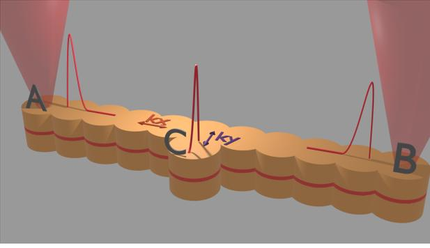
**Figure 1:** Architecture of a logical gate: each micropillar has a few microns diameter, and is composed of a cavity formed by a top and a bottom Bragg mirror with an active medium (red) composed of gain and saturable absorber quantum wells (see [24] for details). Input pulses are sent at each extremities (A and B) of a lattice of coupled micropillars with a coupling factor  $\kappa_x$ . The output pillar (C) is coupled to the middle of the chain with a coupling factor  $\kappa_y$ .
