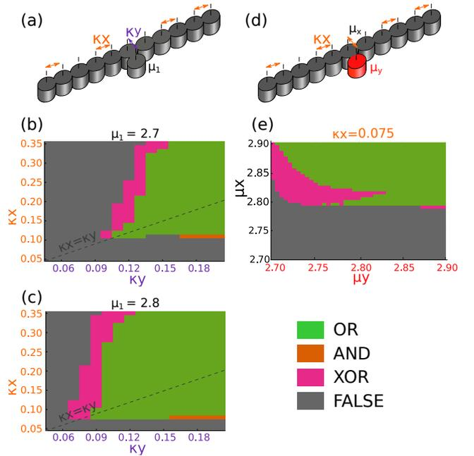
**Figure 5:** Nature of the logical gate for different parameters: uniform pumping but different  $\kappa_x$  and  $\kappa_y$  for (b) and (c) [schematic in (a)] uniform coupling ( $\kappa_x = 0.075$ ) but different pumping for cavity C [in (e), schematic in (d)].
