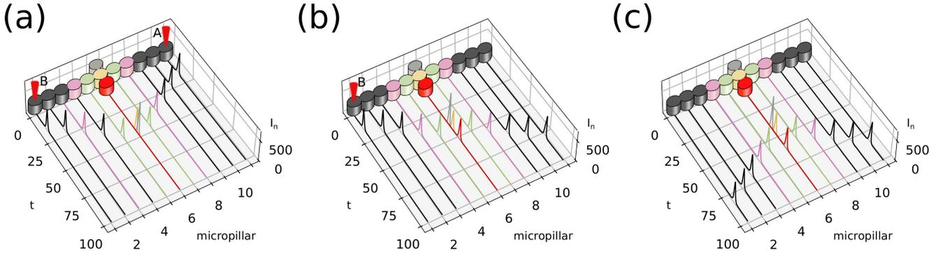
**Figure 6:** NAND gate : (a) architecture with  $\mu_g = 2.7$ ,  $\kappa_x = 0.15$  and  $\kappa_y = 0.12$ . The overpumped pillar (in gray) is pumped at  $\mu_{g2} = 3.15$ . (b) Propagation in the gate when the two inputs are equal to 0. (c) With one input equal to 1. (d) The two input equal to 0.
