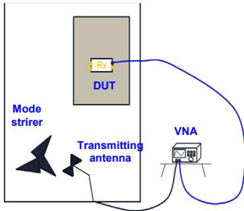
Figure 13: Experimental approach in the MSRC
