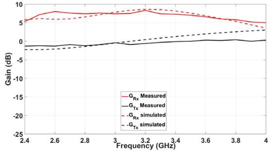
Figure 5: Gains of transmitting and receiving antennas
