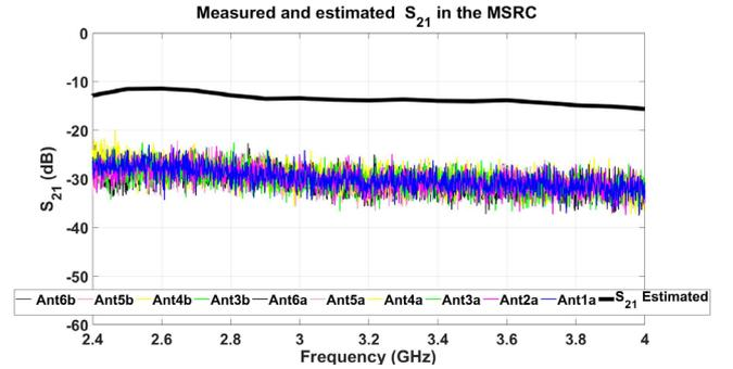
Figure 15: Maximum value of  $S_{21}$  between the transmitting antenna and patch antennas on the DUT in the MSRC
