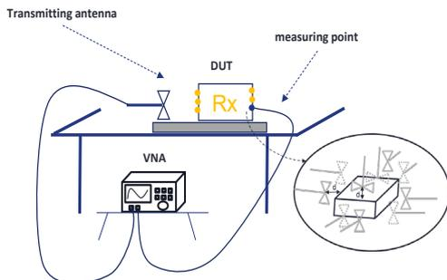
Figure 8: experimental approach in the NFT
