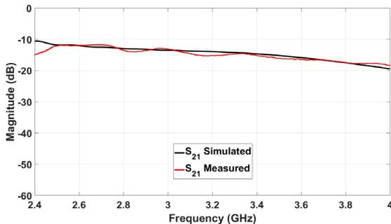
Figure 6:  $S_{21}$  parameters comparison in free space
