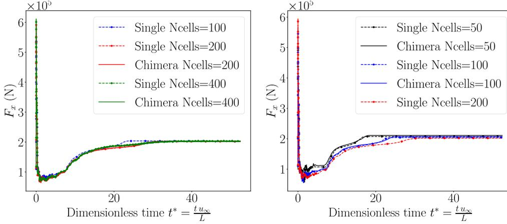
**Figure 15:** Time history of the pressure drag force for several number of grid cells ( $N_{cells}$ ) obtained on both the single-grid configuration, and the overlapping grids with however similar grid spacings ( $\chi = 1$ ).
