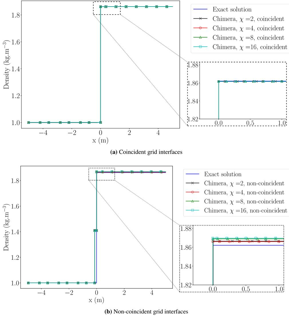
**Figure 11:** Density profile of the stationary shock converged solution in a Chimera configuration with coincident and non-coincident grids for  $N_{cells} = 25$  and  $\chi$  varying from 2 to 16 compared to the exact solution.
