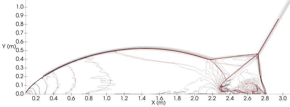
**Figure 31:** Density contours obtained with the present Chimera approach (black iso-contour lines) by using  $N_{cells} = 80$  cells on the substrate and a cell ratio  $\chi = 8$  on the patch, compared to the single mesh case (red iso-contour lines) with  $N_{cells} = 640$ , at an equivalent dimensionless time  $t^* = 0.2 + t_0^*$ . 30 density contours from  $\rho = 1.4$  to 21.4.
