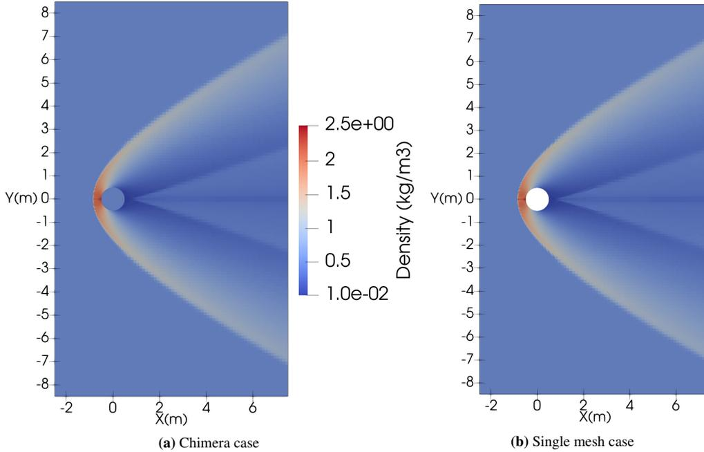
**Figure 14:** Steady state density field for both single grid case (on the left), and the overlapping grids (on the right) with a cell ratio of unity ( $\chi = 1$ ), obtained at a dimensionless time  $t^* = 52$  and for  $N_{cells} = 200$  grid cells along the cylinder perimeter.
