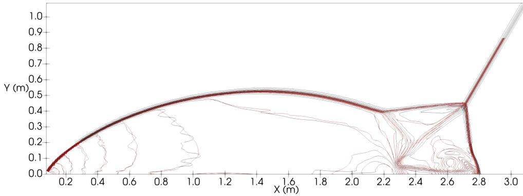
**Figure 29:** Density contours obtained with the present Chimera approach (black iso-contour lines) by using  $N_{cells} = 80$  cells on the substrate and a cell ratio  $\chi = 2$  on the patch, compared to the single mesh case (red iso-contour lines) with  $N_{cells} = 160$ , at an equivalent dimensionless time  $t^* = 0.2 + t_0^*$ . 30 density contours from  $\rho = 1.4$  to 21.4.
