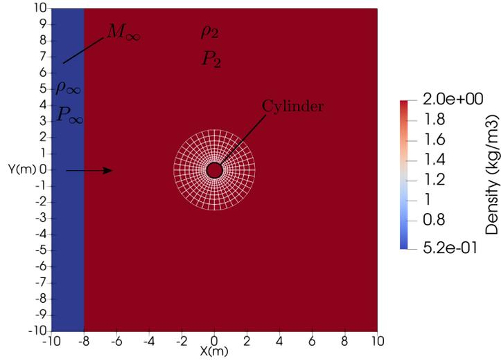
**Figure 12:** The circular cylinder test case: computational domain and the initial solution.
