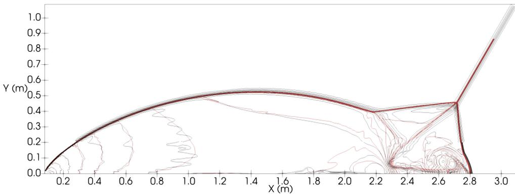
**Figure 30:** Density contours obtained with the present Chimera approach (black iso-contour lines) by using  $N_{cells} = 80$  cells on the substrate and a cell ratio  $\chi = 4$  on the patch, compared to the single mesh case (red iso-contour lines) with  $N_{cells} = 320$ , at an equivalent dimensionless time  $t^* = 0.2 + t_0^*$ . 30 density contours from  $\rho = 1.4$  to 21.4.
