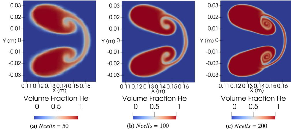
**Figure 24:** Helium volume fraction field obtained with the present Chimera method with overlapping grids with the same cell ratio ( $\chi = 1$ ) at  $t^* = 1.54$ , for a number of cells along the bubble diameter of  $N_{cells} = 50$  (on the left), 100 (in the middle), and 200 (on the right).
