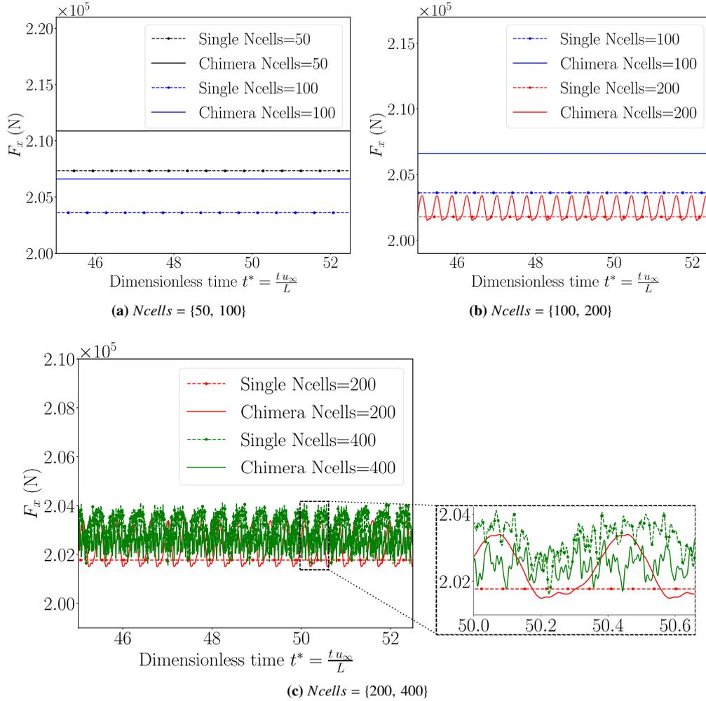
**Figure 16:** Zoom in the interval dimensionless times  $t^* \in [45 ; 52.5]$  of the pressure drag force history for several number of grid cells ( $N_{cells}$ ), obtained on both the single-grid configuration, and the overlapping grids with however similar grid spacings ( $\chi = 1$ ).
