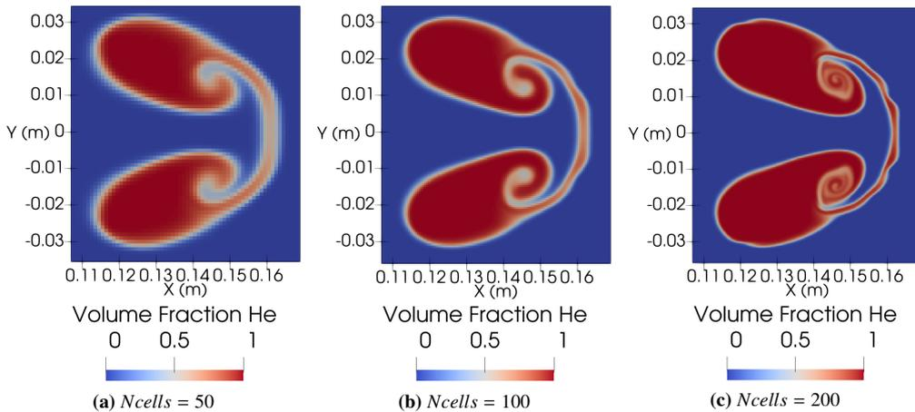
**Figure 23:** Helium volume fraction field obtained in the single mesh case at  $t^* = 1.54$ , for a number of cells along the bubble diameter of  $N_{cells} = 50$  (on the left),  $100$  (in the middle), and  $200$  (on the right).
