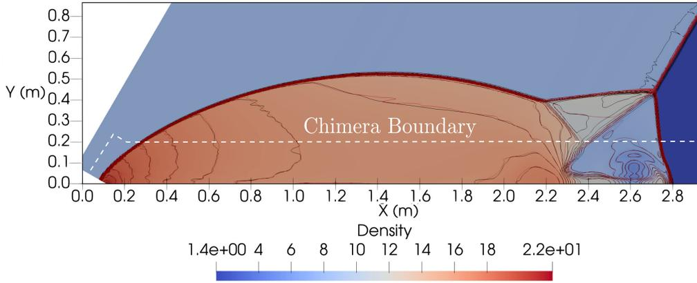
**Figure 28:** Density contours obtained with the present Chimera approach (black iso-contour lines) compared to the single mesh case (red iso-contour lines) at an equivalent dimensionless time  $t^* = 0.2 + t_0^*$  for  $N_{\text{cells}} = 160$  and  $\chi = 1.0$ . 30 density contours from  $\rho = 1.4$  to 21.4. Dashed white line materializes the patch boundary.
