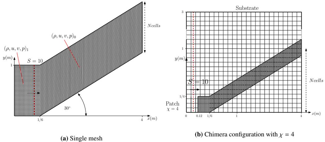
**Figure 27:** Computational domains and initial conditions: configurations of the single mesh case (a), and the Chimera case (b) displayed with a cell ratio  $\chi = 4$ .
