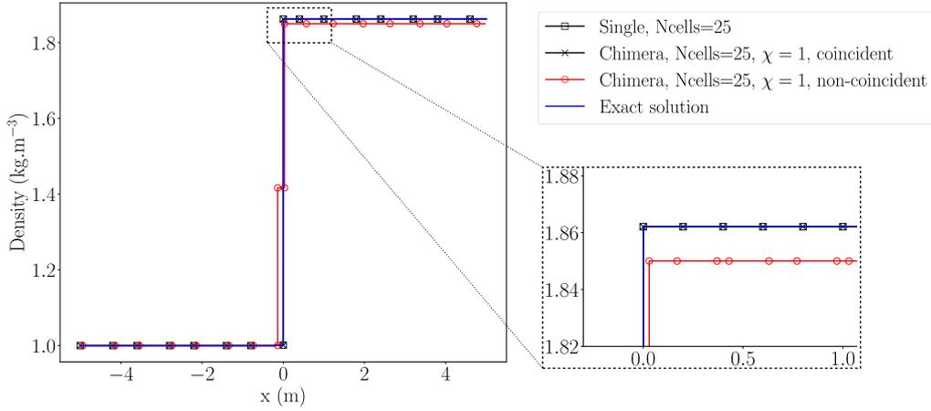
**Figure 10:** Density profile of the stationary shock converged solution in a single grid configuration with  $N_{cells} = 25$  and a Chimera configuration with coincident and non-coincident grids for  $N_{cells} = 25$  and  $\chi = 1$  compared to the exact solution.
