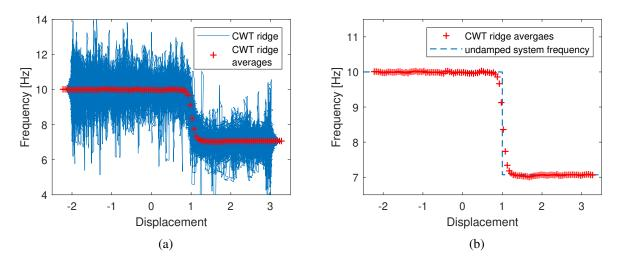
Figure 5: Numerical simulations, second case study: (a) CWT ridge  $f_r$  as a function of displacement x (blue), with its averages by displacement increments of 0.05 (red), (b) CWT ridge averages (red), and undamped system frequency  $\tilde{\omega}/2\pi$  (blue).
