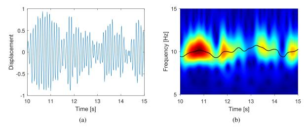
Figure 3: Numerical simulations, first case study: (a) extract of the system response x, (b) modulus of its CWT, with associated ridge (black curve).
