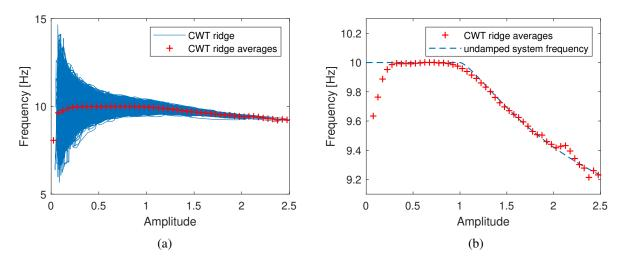
Figure 4: Numerical simulations, first case study: (a) CWT ridge  $f_r$  as a function of its amplitude  $A_r$  (blue), with its averages by amplitude increments of 0.05 (red), (b) CWT ridge averages (red), and undamped system frequency  $\tilde{\omega}/2\pi$  (blue).
