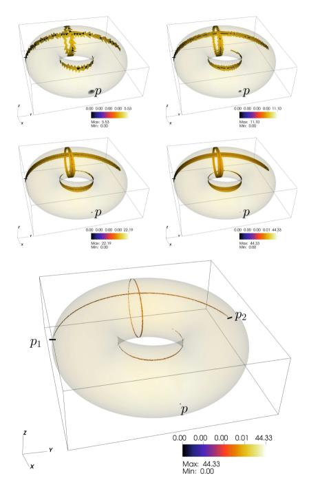
FIGURE 3. Numerical identification of the  $C_{p,h,\epsilon}$  of a torus obtained at four uniform mesh refinement levels for  $\epsilon=0.001$ . The color map refers to  $\mu_h^*$  values. The coarsest mesh level contains 2712 nodes and 5424 triangles. The two segments in black intersect the surface of the torus at points  $p_1$  and  $p_2$  described in Figure 1. The bottom panel shows the  $C_{p,h,\epsilon}$  for  $\epsilon=0.0001$  on the finest grid level.
