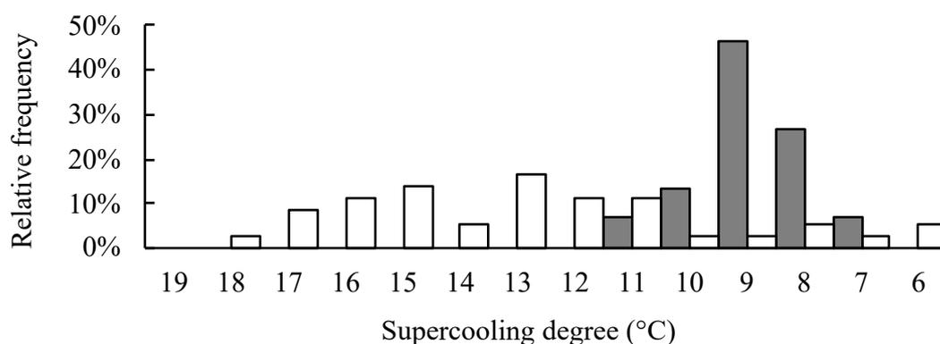
**Fig. 3.** Supercooling relative frequency for scaffolds freeze-dried in spaced configuration (white bars) and contiguous configuration (gray bars). In the latter case, scaffolds are in packs of 50 contiguous scaffolds. Crosslinker feed ratio  $r = 96 \text{ mol mol}^{-1}$ .
