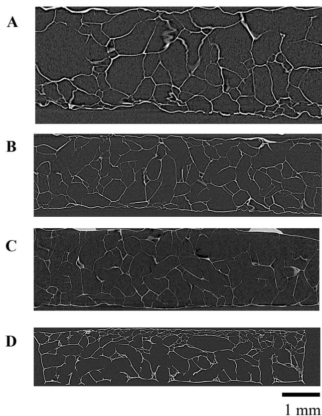
**Fig. 5.** XZ slices of freeze-dried hydrogel scaffolds acquired by X-ray tomography with 6- $\mu\text{m}$  resolution. The supercooling degree (during freeze-drying) was set at  $10 \pm 0.2^\circ\text{C}$ . Crosslinker feed ratio  $r = 48 \text{ mol mol}^{-1}$  (**A**),  $r = 72 \text{ mol mol}^{-1}$  (**B**),  $r = 96 \text{ mol mol}^{-1}$  (**C**), and  $r = 161 \text{ mol mol}^{-1}$  (**D**). Scale bar stands for 1 mm. The slices A to C are not whole in X-direction.
