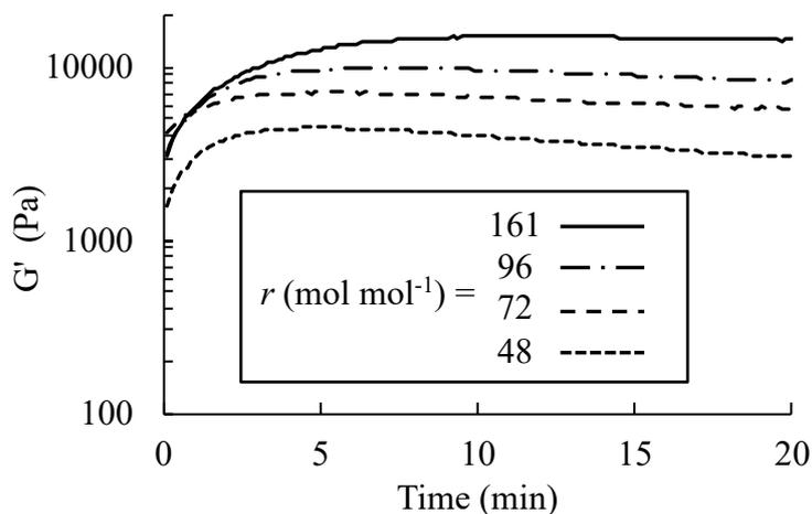
**Fig. 1.** Variations of the storage modulus at 1 Hz during crosslinking at 50°C. Crosslinker feed ratio  $r = 48$  mol mol<sup>-1</sup> (dotted line), 72 mol mol<sup>-1</sup> (dashed line), 96 mol mol<sup>-1</sup> (dash-dotted line), 161 mol mol<sup>-1</sup> (continuous line).
