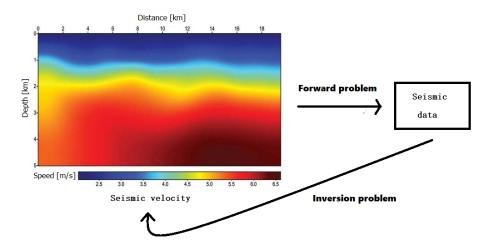
Fig. 1. Illustration of the seismic inversion problem.
