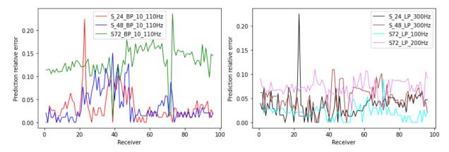
**Fig. 17.** P-wave label prediction relative errors for different sources at all receivers and for different frequency filters: 10-110 Hz band-pass filter (left), for 100, 200 or 300 Hz low-pass filters (right). The predicted errors are low and acceptable except close to the sources due to near-wave field issues.
