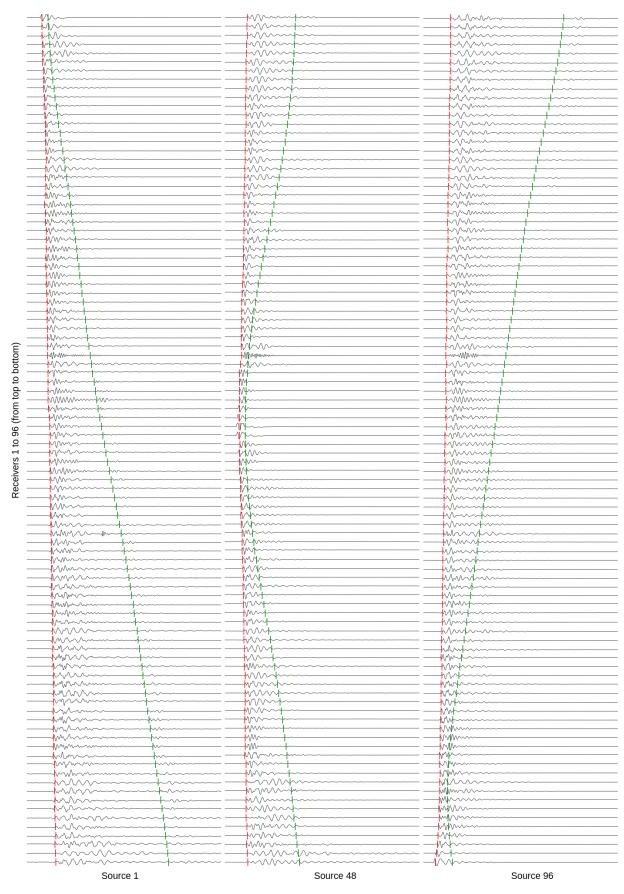
**Fig. 13.** Seismograms for sources 1 (picked by hand), 48 (labeled using semi-supervised learning) and 96 (picked by hand). The labels of first arrival times are shown (red) and are detected for all seismograms. This is not the case for the surface (Rayleigh) train-waves (green) which are detected very far from the sources because only one component is recorded at all receivers.
