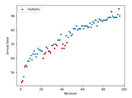
**Fig. 9.** Outlier detection of P-wave pseudo-labels (time arrivals normalized by the 0.5 ms sampling time step) for the leftmost located source (i.e. source 1) using Huber logarithmic regression, where  $\epsilon = 1.55$  is a threshold controlling the number of samples that should be classified as outliers.
