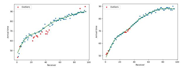
Fig. 12. Correcting P-wave pseudo-labels (time arrivals normalized by the 0.5 ms sampling time step) at iteration 1 (left) and at iteration 5 (right) using SVR, where the maximum error  $\epsilon = 0.1$  and the regularization parameter C = 200.
