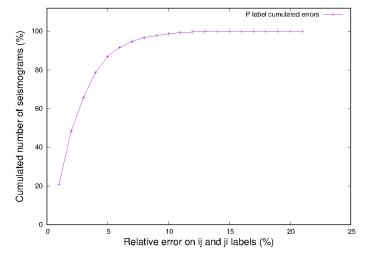
**Fig. 16.** Cumulated relative errors of the differences of picked labels between (i, j) and (j, i) source-receiver pairs for the P-wave. The relative errors of the picked P-labels are smaller than 6% over almost 96% of the global dataset of seismograms.
