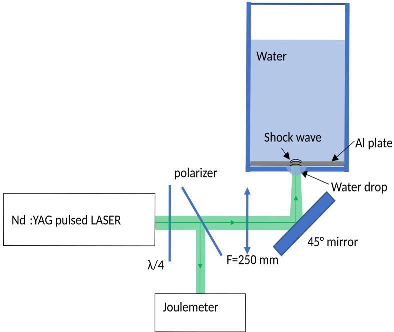
Figure 11: Experimental setup used to create flat bubbles.
