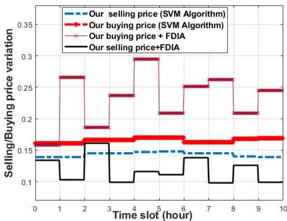
FIGURE 6. The SVM performance in extracting the right price value (buying and selling) after FDIA.
