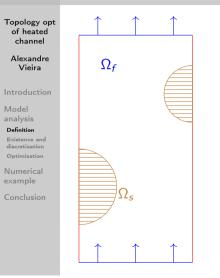
In a region  $\Omega$ , suppose a flow occupies a region  $\Omega_f$  and the solid defines a region  $\Omega_s$  such that  $\Omega = \Omega_f \cup \Omega_s$ . Suppose also that the channel is heated.
