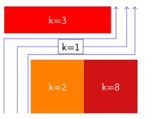
Usually, thermal conductivity = discrete set of constants. We would like to control the distribution of thermal conductivity also!
