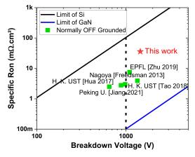
**Figure 6.** Benchmarking of breakdown voltage vs. specific on-resistance of normally off transistors with a grounded substrate. Solid lines in black and blue represent the theoretical limits of Si and GaN, respectively.
