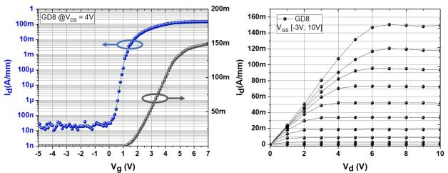
**Figure 4.** Transfer (**left**) and output (**right**) characteristics of a p-GaN/AlGaN/GaN HEMT with a gate–drain distance of 8  $\mu$ m at V<sub>DS</sub> = 4 V plotted in semi-log and linear scale.
