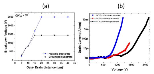
**Figure 5.** Three-terminal breakdown voltage at  $V_{GS} = 0$  V of p-GaN/AlGaN/GaN HEMTs with floating and grounded substrate: (a) as a function of the gate-to-drain distance and (b) for various gate-to-drain distances.
