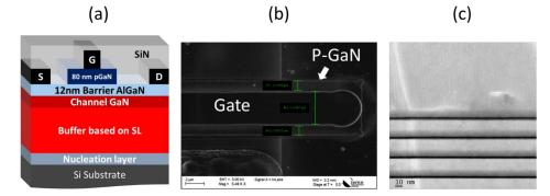
**Figure 1.** (a) Schematic cross section of the p-GaN/AlGaN/GaN HEMT on Si. (b) SEM top view of the gate including the partially etched p-GaN layer and (c) a zoomed TEM image of the superlattices.
