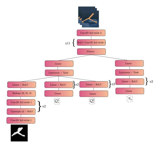
Figure 8: SGQN neural network architecture
