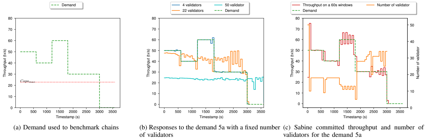
Fig. 5. Comparison of committed throughput for a common demand for chains with and without Sabine
