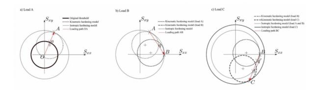
Fig 1. Schematic representation of strain hardening effects on the elastic threshold during the loading process. a)
