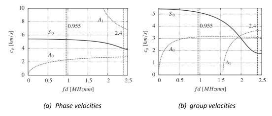
Figure 1. Dispersion curves of 2mm aluminum plate showing (a) phase and (b) group velocities of the antisymmetric modes  $(A_i)$  'dashed' and the symmetric modes  $(S_i)$  'continuous' [2]
