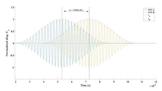
Figure 3. Normalized analytical displacement  $U_z$  at points A and B with  $t_{c_{ana}}$
