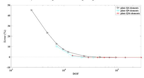
Figure 4. Convergence of different plate element types according to the degrees of freedom
