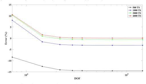
Figure 7. The effect of the number of timesteps (timestep estimate) on the convergence value
