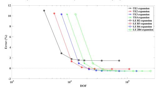
Figure 5. Convergence analysis of the different out of plane expansions according to the degrees of freedom
