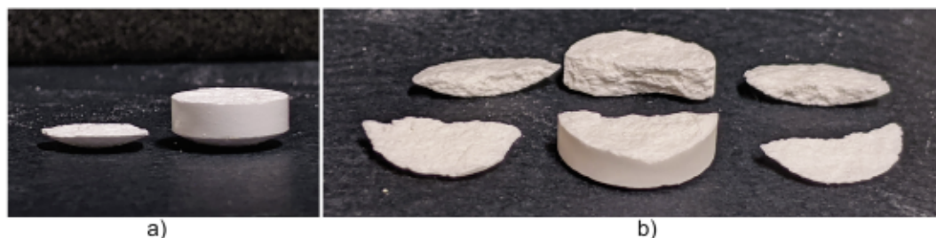
Fig. 1. Examples of capped tablets characterized a) out-of-the die and b) after the diametral test (both cups came off).
