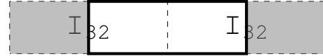
(a) Fetching the bottom half of a 32-bit instruction and the top half of another 32-bit instruction.
