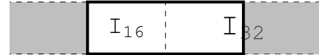
(b) Fetching one 16-bit instruction and the top half of a 32-bit instruction.
