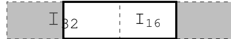
(c) Fetching the bottom half of a 32-bit instruction and one 16-bit instruction.
