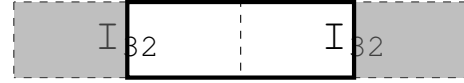
(a) Fetching the bottom half of a 32-bit instruction and the top half of another 32-bit instruction.
