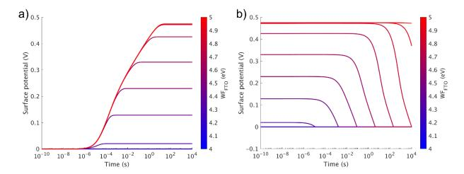
Figure 9: Perovskite -  $TiO_x$  transient SPV simulations for different values of the back contact work function ( $WF_{FTO}$ ); build-up of SPV after illumination is switched on (a), and SPV decay after illumination is switched off (b).
