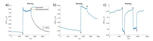
Figure 4: KPFM measurements performed on perovskite-SCTL structures, under 532 nm laser illumination. CPD measurement of (a) perovskite-TiO<sub>x</sub>, (b) perovskite-SnO<sub>x</sub>, and (c) perovskite-NiO<sub>x</sub>. Arrows indicate switch on and subsequent switch off times of the 532 nm laser illumination.
