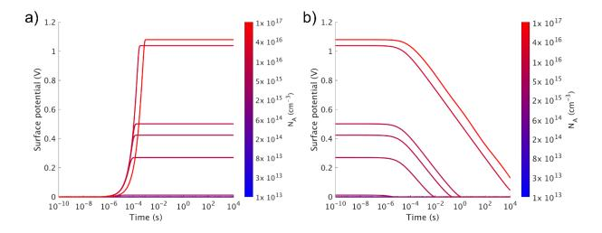
Figure 6: Perovskite - TiO<sub>x</sub> transient SPV simulations for different values of acceptor dopant concentration in the perovskite; build-up of SPV after illumination is switched on (a), and SPV decay after illumination is switched off (b).
