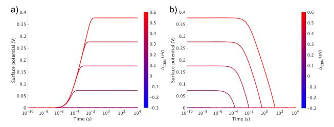
Figure 7: Perovskite - TiO<sub>x</sub> transient SPV simulations for different values of conduction band offset.  $\Delta E_{\rm C} = E_{\rm C,pvk} - E_{\rm C,TiO_x}$ ; build-up of SPV after illumination is switched on (a), and SPV decay after illumination is switched off (b)
