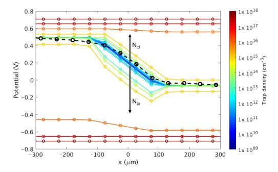
Figure 3: Surface potential of the MAPbI<sub>3</sub> perovskite across the LHJ device convoluted with the 200  $\mu m$  collection diameter of the XPS setup employed, for different trap (shallow donor  $N_{td}$  or shallow acceptor  $N_{ta}$ ) concentrations in the perovskite. The dark dashed line represents the experimental data.
