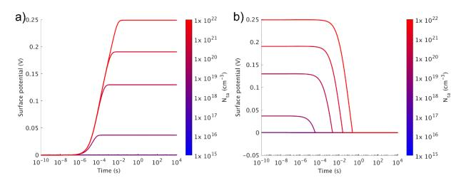
Figure 8: Perovskite -  $TiO_x$  transient SPV simulations for different values of acceptor trap density on a 5 nm layer thickness on the surface of  $TiO_x(N_{ta})$ , close to the interface with the perovskite: SPV rise (a) and decay (b) after illumination is switched off.
