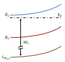
Figure 1: Sketch of the  $I_{3d_{5/2}}$  core level, top of the valence band,  $E_V$ , and bottom of the conduction band,  $E_C$ , in presence of a space-dependent electrostatic potential,  $q\varphi(x) = BE_I(x) = E_F - I_{3d_{\frac{5}{2}}}(x)$ .
