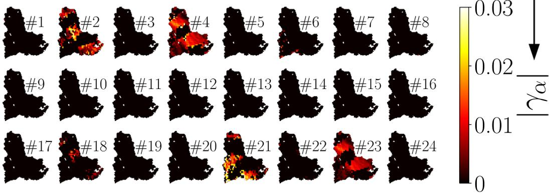
Figure 8: Illustration of kinematics identification of slip activity at  $E_{x,U} = 2.09\%$  in a given grain: (a) In-plane components of displacement gradient tensor  $\underline{H}$  measured with Digital Image Correlation. (b) Projected displacement gradient  $H_\alpha$  for every slip system  $\alpha$  (see Tab. 2). (c) Plastic shear by slip  $\gamma_\alpha$  that allows for identification of active slip systems. It is computed after projected displacement gradient  $H_\alpha$ .
