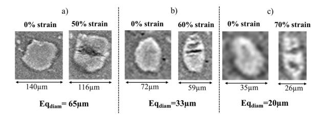
Figure A6: The smallest  $CB_{aggl}$  that undergo fracture at a given strain. a)  $CB_{aggl}$  with  $Eq_{diam} = 65\mu m$  undergo fracture at 50% nominal strain. b)  $CB_{aggl}$  with  $Eq_{diam} = 33\mu m$  undergo fracture at 50% nominal strain. c)  $CB_{aggl}$  with  $Eq_{diam} = 20\mu m$  undergo fracture at 50% nominal strain.
