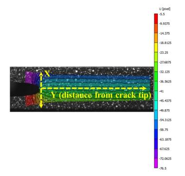
Figure A5: Example of displacement field  $(U_x)$  along the tensile direction deduced from DIC measurement during crack propagation.
