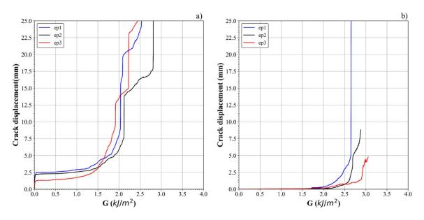
Figure A1: Crack displacement as a function of G for a) F2 and b) F3.
