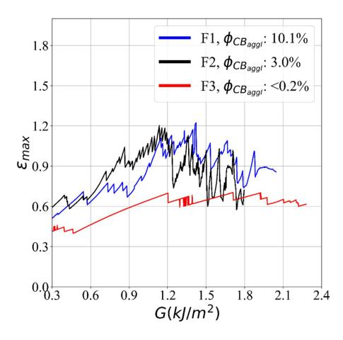
Figure 7:  $\epsilon_{max}$  observed next to crack tip as a function of G for F1, F2 and F3,
