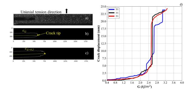
Figure 2: a) Stretched notched PS specimen with speckled pattern. b) Crack contour plotted derived from the picture (a) at a given G. The yellow star denotes the crack tip c) evolution of the crack contour after the increase of G by  $0.2kJ/m^2$ . d) Crack displacement measured with three specimens of the same model material F1 as a function of G. The same plots for F2 and F3 materials are reported in SI (Figure A1).
