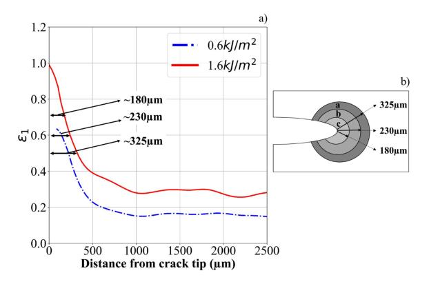
Figure 12: a) Nominal strain profile ahead of the crack tip) for F1 at 2 G values ( $0.6 \text{ kJ/m}^2$ ,  $1.6 \text{kJ/m}^2$ ). The arrow indicates the size of the zone for which the nominal strain is above 50%, 60%, and 70%. The plot for F2 is presented in SI (Figure A9). b) Scheme of the influence zone
