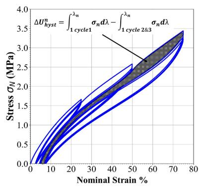
Figure A4: Materials have been cyclically deformed three times up to a fixed nominal strain
