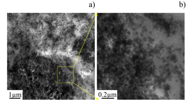
Figure 3: a) TEM image of a slice of  $CB_{aggl}$  in F1 at a resolution of 1µm, b) zoomed portion of the yellow square in 'a)' at a resolution of 200nm.
