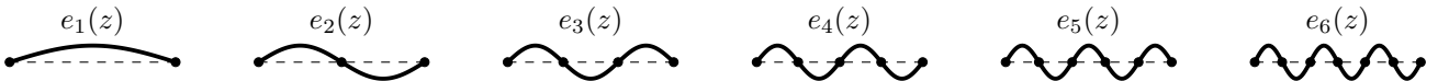
Figure 2: First 6 eigenmodes e_n(z) of the linear string of length L . The nodes (stationary points) are indicated by dots.
