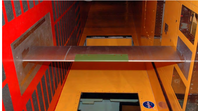
Fig. 10 36-inch NACA23012 Airfoil in icing tunnel (rotated) [4].
