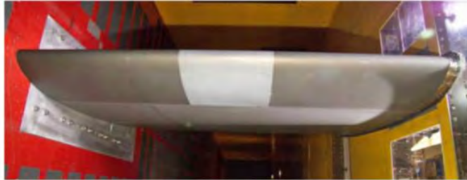
Fig. 15 72-inch NACA23012 Airfoil in icing tunnel (rotated) [5].
