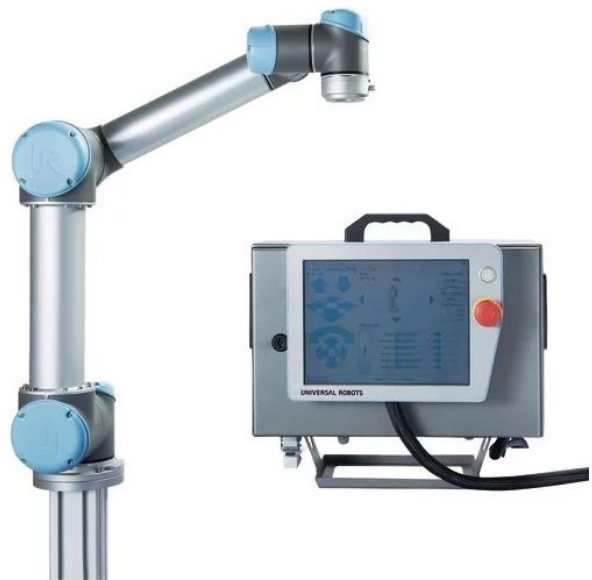
Figure 1: Picture of a UR robot and its teach pendant
