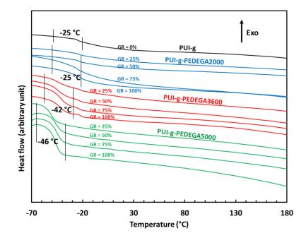
Fig. 3 Thermograms of PUI-g and grafted PUI multi-block copolymers with different lengths of grafts (PEDEGA 2000, 3600 and 5000) and different grafting rates (GR) from 25 to 100% (second heating – 10°C/min). Note: The thermograms have been shifted for improved visualization and correspond to arbitrary heat flow values.
