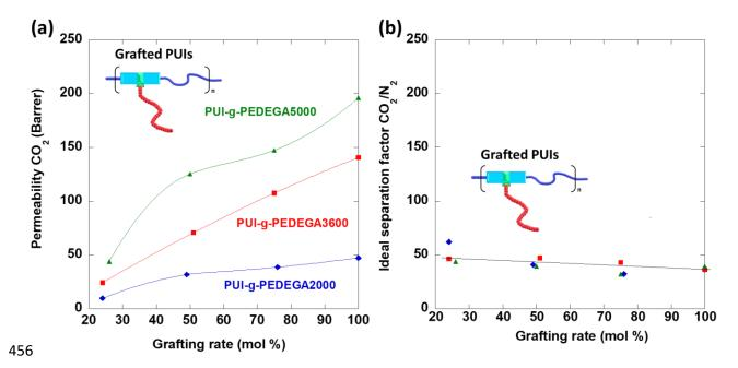
457 Fig. 8. Influence of grafting rate on (a) permeability of CO<sub>2</sub> and (b) ideal separation factor αCO<sub>2</sub>/N<sub>2</sub> for the grafted
