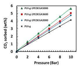
Fig. 7. Influence of soft grafts molecular weight on CO<sub>2</sub> sorption isotherms of the PUI copolymers grafted with maximum grafting rate (100%) and their precursor PUI-g at 35°C.
