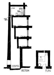
Cut & plan of the traditional system of the feaces chamber – ©Fernando Varanda
