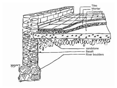
A typical section of foundation, wall and ground floor- after Miles & Ahmet
