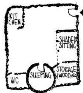
Round reed house layout in high-walled yard – ©Fernando Varanda
