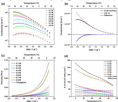
conductivity recorded on a 0.5 M Ca(TFSI)<sub>2</sub>/G4 solution. (c) Temperature dependence of the viscosity of Ca(TFSI)<sub>2</sub>/G4 solutions at different
