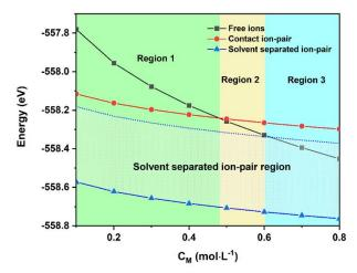
**Figure 3.** Concentration-dependent free enthalpy of: Free *mer*- $[Ca(G4)_2]^{2^+}$  and TFSI $^-$  (Black line), Contact ion-pair *trans*- $[Ca(\mu_2-TFSI)(G4)]^+$  with a G4 molecule in its second solvation shell (Red
