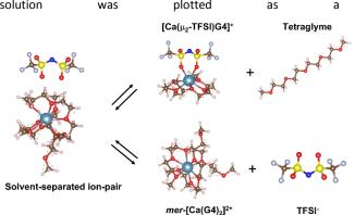
**Figure 2.** Molecular representation of  $[mer-[Ca(G4)_2]]/[TFSI]^+$  solvent-separated ion-pair and its evolution to trans- $[Ca(\mu_2-TFSI)(G4)]^+$  contacting ion-pair and free ions.
