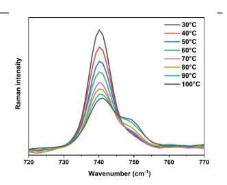
**Figure 5.** Evolution in the position and the intensity of the characteristic expansion-contraction mode of TFSI<sup>-</sup> at 740 cm<sup>-1</sup> during the temperature-dependent in situ Raman measurement performed on a 0.1 M Ca(TFSI)<sub>2</sub>/G4 solution.
