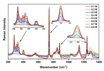
**Figure 4.** Raman spectra acquired on  $Ca(TFSI)_2/G4$  solutions at different salt concentrations. Insets focus on the zoom of some important vibrational modes.
