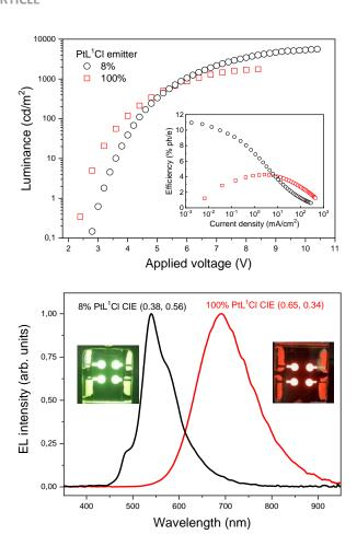
**Figure 4** a) Luminance vs applied voltage and external EL efficiency vs current density (inset) of the OLEDs. b) Electroluminescence spectra at 7 V of OLEDs. In the inset there are photos of yellow-green and deep red OLEDs based on [PtL<sup>1</sup>Cl].
